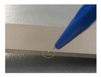
• a burr on the underside of the cut-out contour
