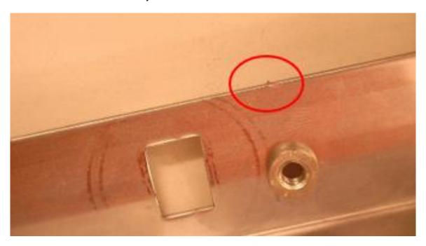
Possibility of visible scratches on the sheet metal surface (the scratches do not affect the product's functionality)
